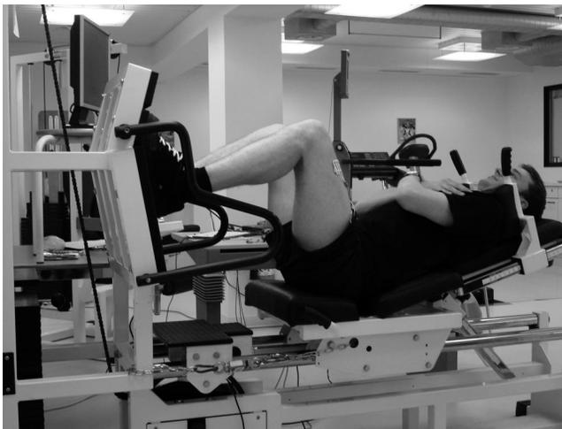
Fig. 2. The horizontal leg press machine equipped with the strain gauge.
